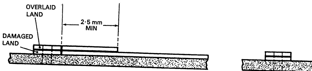
Figure 7 REPAIR OF DAMAGED LAND—OVERLAID LAND
